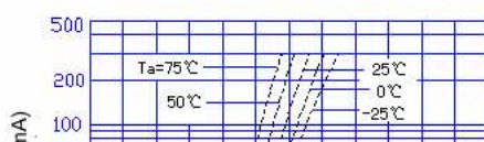
Fig. 1 Forward current vs Forward voltage
